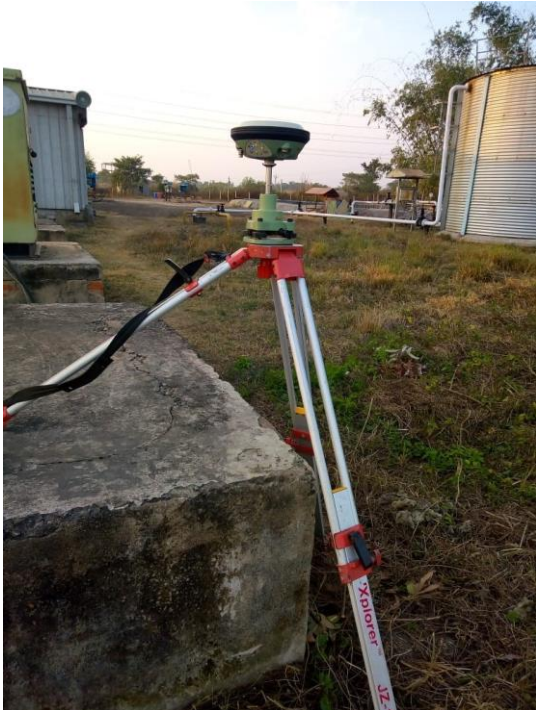
Plate 1: Subsidence monitoring station at ES5A
