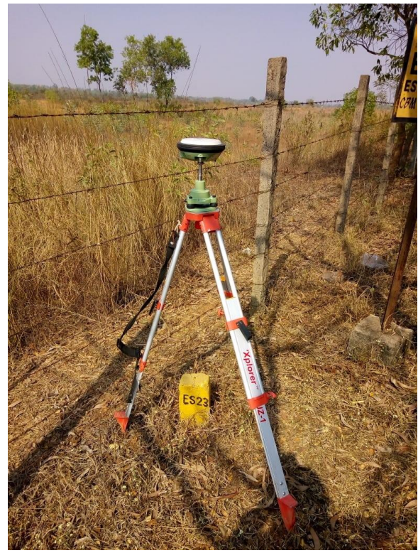
Plate 6: Subsidence monitoring station at ES23
