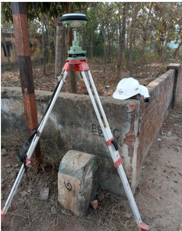
Plate 3: Subsidence monitoring station at ES15C
