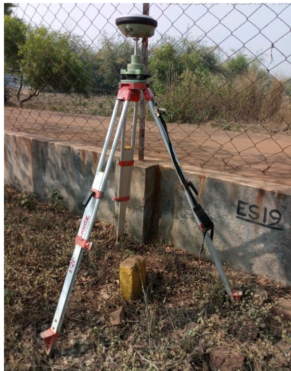
Plate 4: Subsidence monitoring station at ES19
