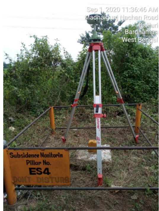
Plate 2: Subsidence monitoring station at ES4
