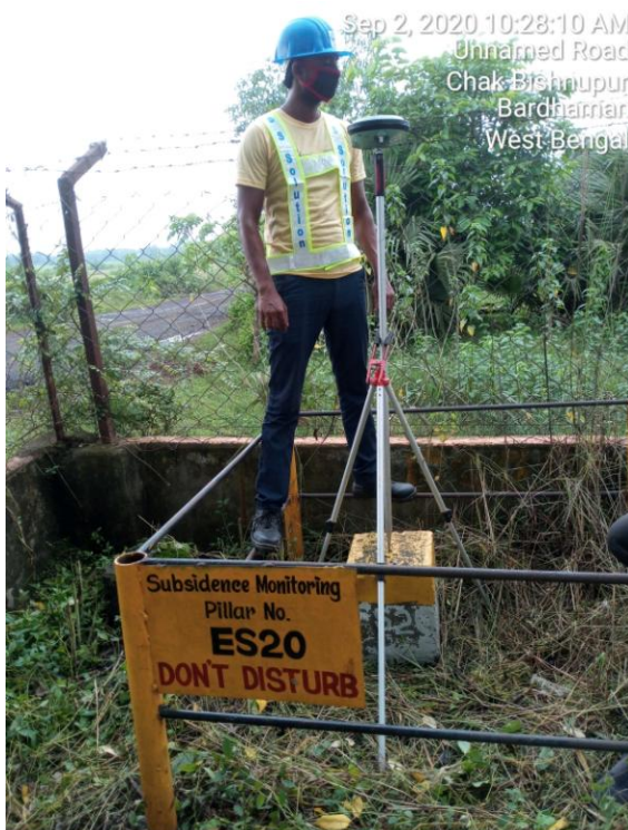
Plate 3: Subsidence monitoring station at ES20
