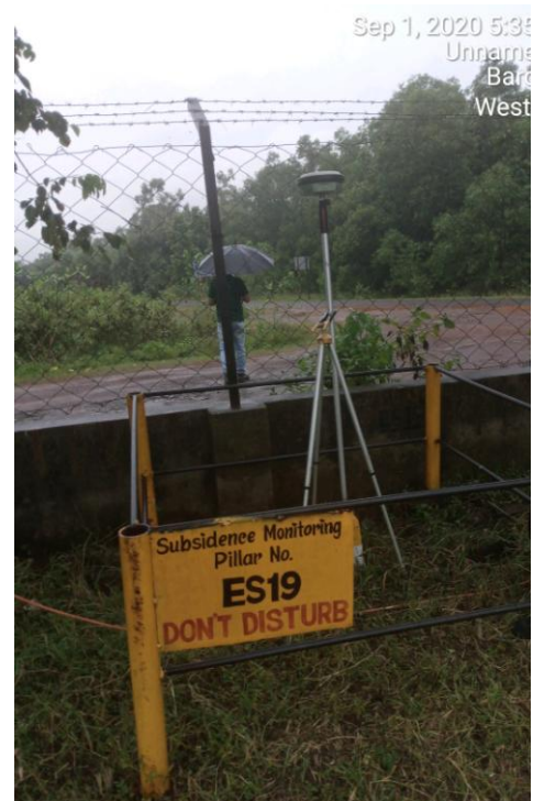
Plate 4: Subsidence monitoring station at ES19
