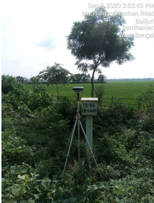
Plate 1: Subsidence monitoring station at ES8N
