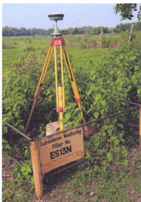
Plate 5: Subsidence monitoring station at ES13N
