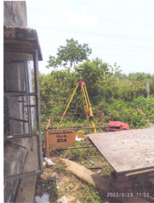
Plate 2: Subsidence monitoring station at ES4
