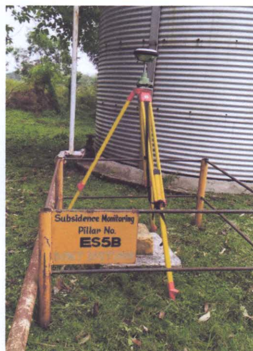
Plate 8: Subsidence monitoring station at ES5B
