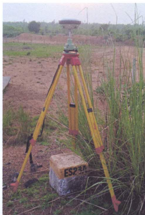
Plate 6: Subsidence monitoring station at ES23A
