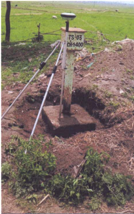
Plate 1: Subsidence monitoring station at ES8N
