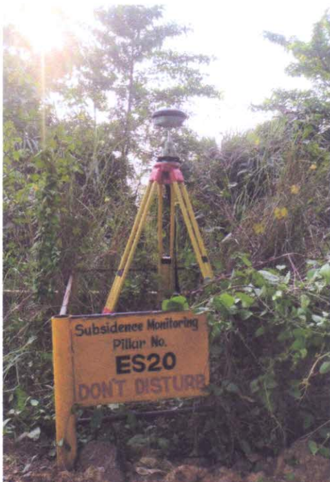
Plate 1: Subsidence monitoring station at ES8N
