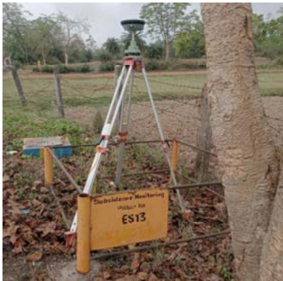
Plate 5: Subsidence monitoring station at ES13
